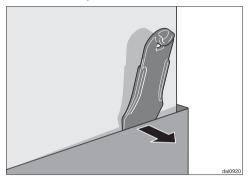
After removing the two screws from the chimney, slide the lever between the chimney and the chimney extension and gently apply pressure to ease the chimney from its hooks.
